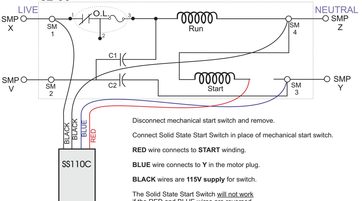
Disconnect mechanical start switch and remove.
